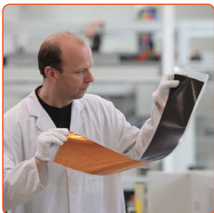
7 flexible super cell in module production. Image courtesy of Odersun
